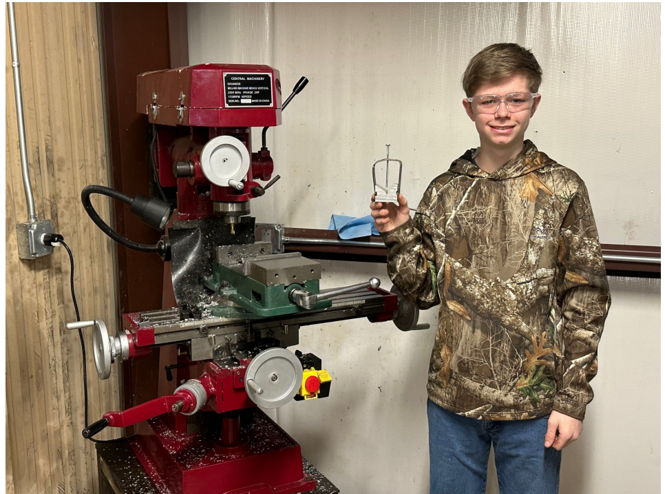
Jacob Kane 90 degree clamp. Created on the milling machine. Also, a tap and die set was learned and used in the process.
